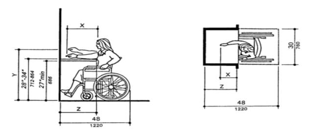
NOTE: x shall be  $\leq$  25 in(635 mm); z shall be  $\geq$  x. When x < 20 in(510 mm), then y shall be 48 in(1220 mm) maximum. When x is 20 to 25 in(510 to 635 mm), then y shall be 44 in(1120 mm) maximum.
