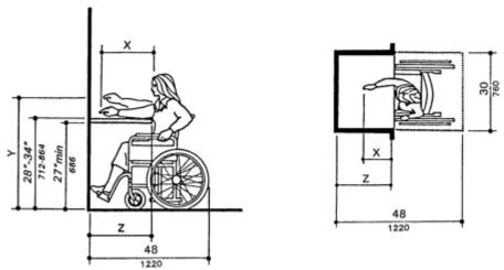
NOTE: x shall be  $\leq$  25 in(635 mm); z shall be  $\geq$  x. When x < 20 in(510 mm), then y shall be 48 in(1220 mm) maximum. When x is 20 to 25 in(510 to 635 mm), then y shall be 44 in(1120 mm) maximum.
