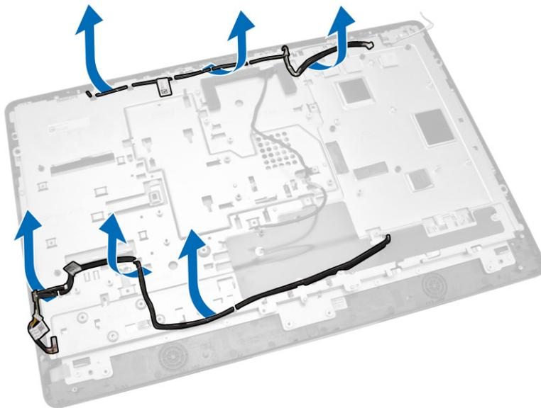
5. Remove the screw that secure WEB GND cable. Remove the tape from both sides of the display panel.
