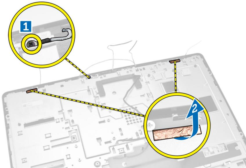
6. Remove the screws that secure the base panel to the chassis. Lift the display-panel base from the display bezel.
