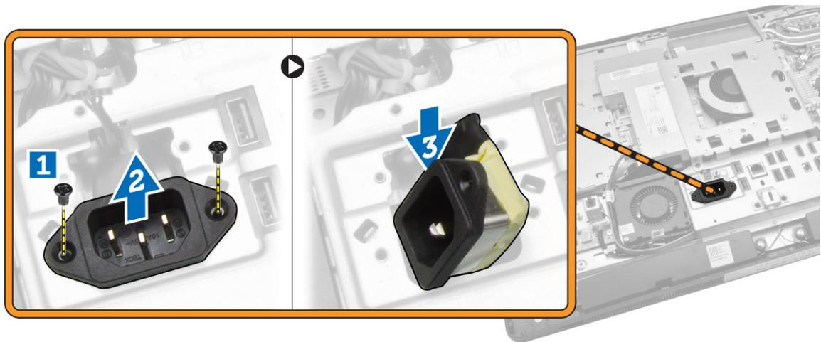
5. Remove the screws that secure the I/O board shield to the chassis. Loosen the power connector and press it down the socket. Flip the input/output (I/O) board shield and remove it from the computer.
