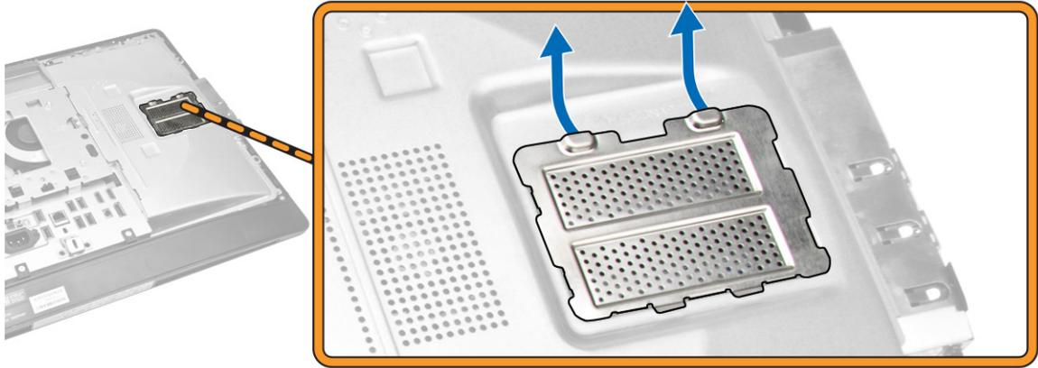
4. Pry the retention clips away from the memory module until it pops-up. Lift and remove the memory module from its connector.
