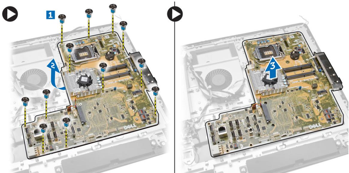
5. Lift and remove the system board from the chassis.
