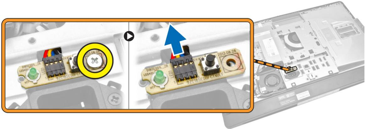
4. Remove the screws that secure the power connector to the I/O board shield.
