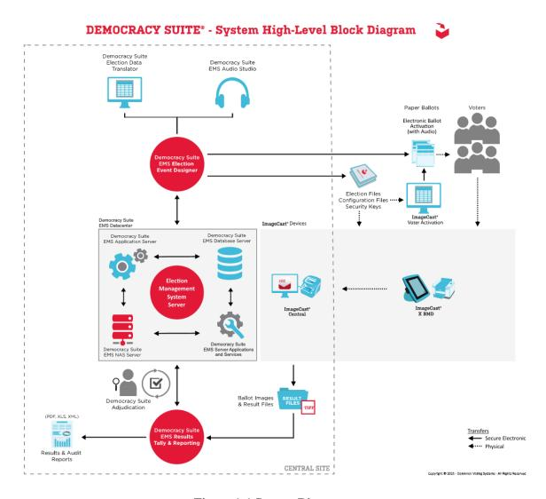
Figure 1-1 System Diagram
