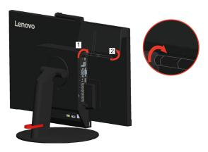
3. Pivot the cable cover as shown to the closed position.
