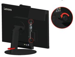
2. Push the computer from the rear as shown to disconnect it completely from the 3 in 1 cable.
