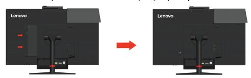
Note: Make sure the Tiny is aligned with the back cover.
