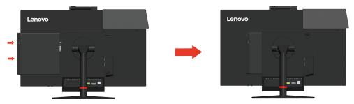
3. Press the computer from the front until it completely snaps into position.
