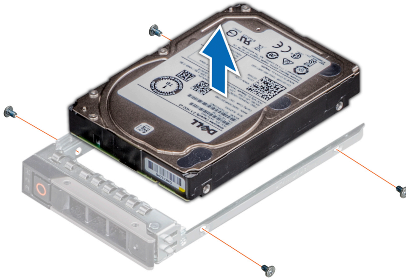
Figure 77. Removing the drive from the drive carrier
