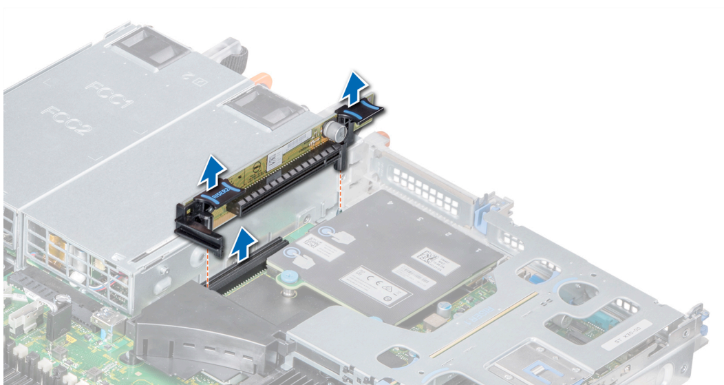
Figure 48. Removing the expansion riser 2A
