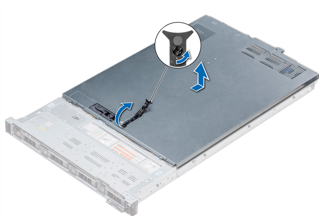
Figure 23. Removing the system cover
