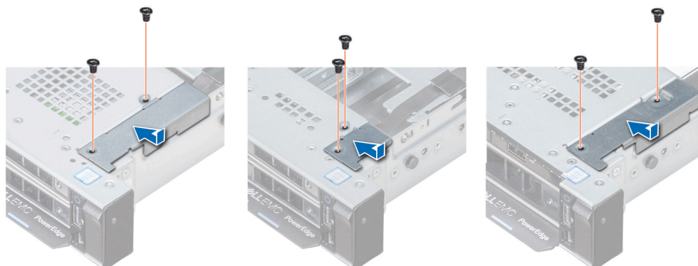
Figure 113. Installing the cable cover
