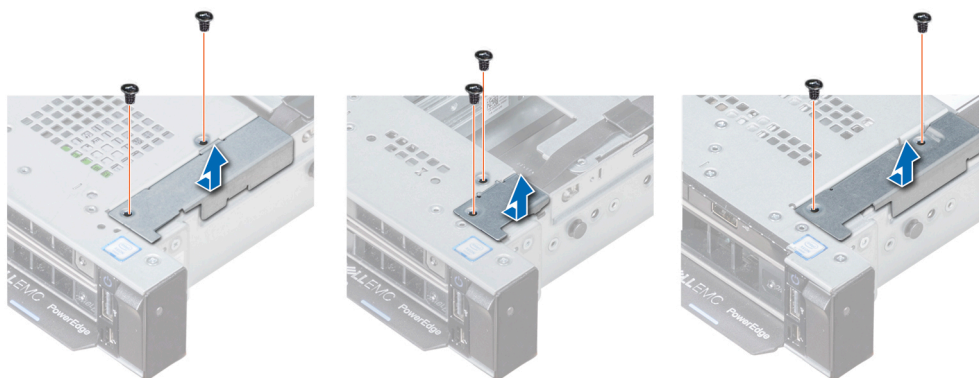
Figure 110. Removing the cable cover
