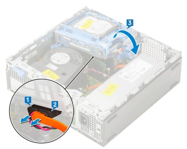
e Push the release latch on the optical drive [1] and pull the optical drive out from the system [3].
