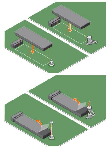
c Place the M.2 Intel optane memory module into the slot on the thermal pad.
