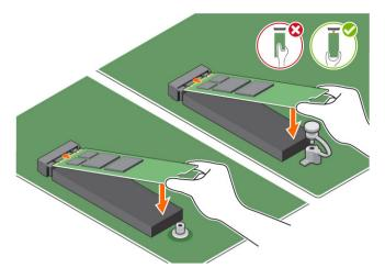
d If the system is shipped with screw tighten that secures the M.2 Intel optane memory module on the computer. If the system is shipped with self locking spacer press to lock the M.2 Intel optane to secure on the computer.
