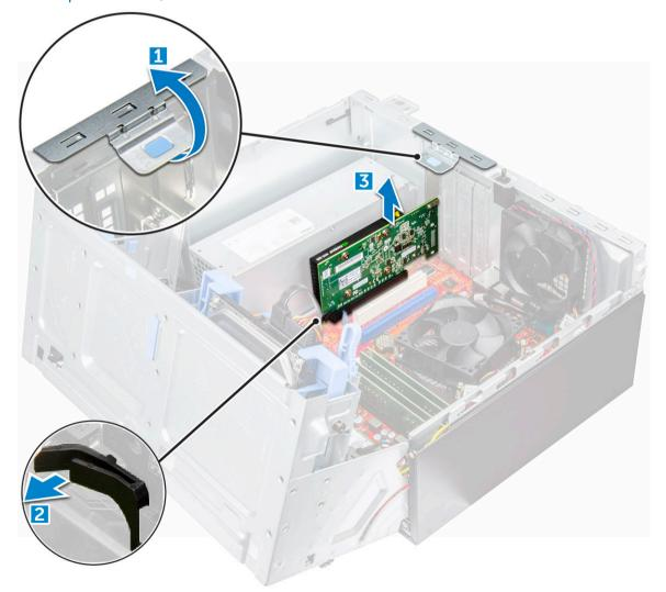
5 Repeat the steps to remove any additional PCIe expansion card.
