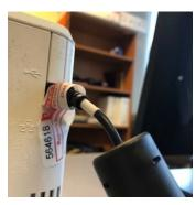
3. Place the second seal over the tail of the first seal and the Ethernet port and log the second seal number.
