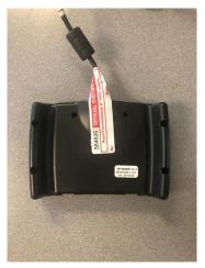
2. With the second seal, wrap around the end of the fist seal that is attached to the cable, make sure that the seal number is visible on both seals.
