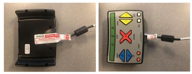
3. ATI USB Cable (ICX Samsung Only) – Seal the USB connection of the ATI Cable to the bottom of the ICX so that the seal covers both ends of the cable.
