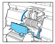
3. Pull the roller lock lever down.
