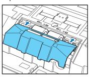
8. Push the front of the retard roller cover in. Make sure to hear a latching sound that it is securely returned to its original position.
