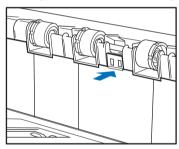
**3.** Open the imprinter cover until it makes contact with the eject tray.
