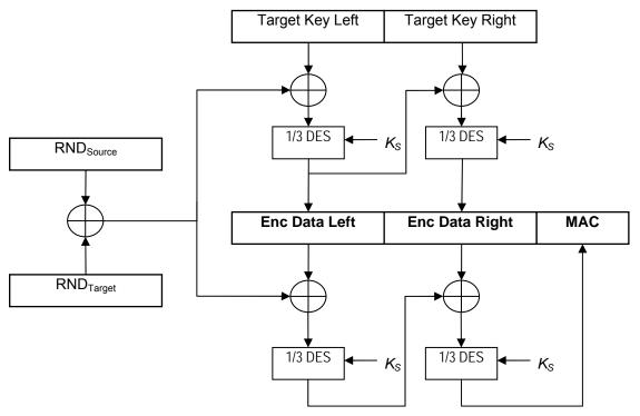
Figure 13: Key injection encryption computation.
