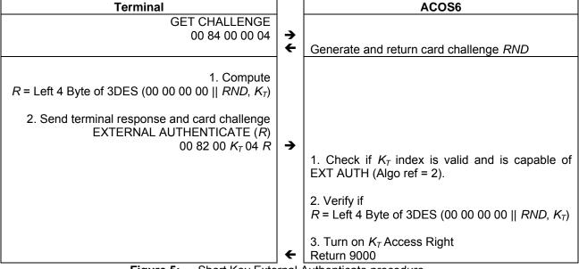
Figure 5: Short Key External Authenticate procedure
