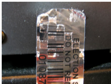
Figure A-2: Evidence of Tampering: Peeled and Reapplied
