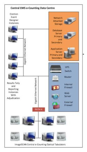
Figure 2-1: Structure of the Central Counting Center
